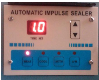
Figure 2. KS-FS Timer Control Panel
